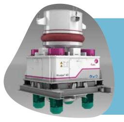
FCB Rhodax®'s selective material bed compression grinding process optimally releases the three components making up concrete - aggregates, sand (0.125-2 mm) and cement paste (0-0.125 mm), which will then be separated and retrieved.
